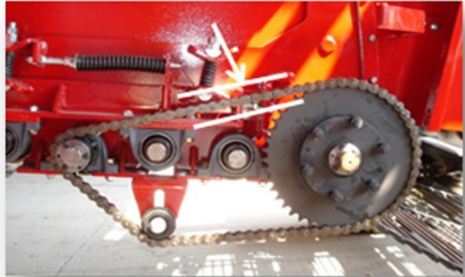
Figure 7-34: Jump Chain Tension
