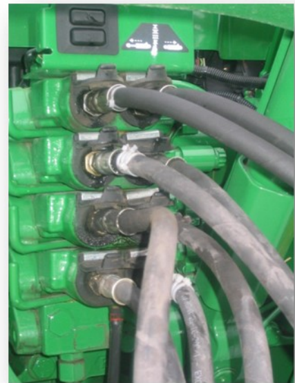
Figure 5-1: Attaching Hydraulic Lines
